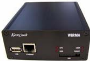
1. Version Telemetry (GSM, GPRS, WLAN) 2. Version Nomad (GSM, GPRS, WLAN et GPS )
